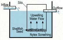
What does our upweller look like? It is a large 3 x 12-foot tank set up with a pump system that brings fresh flowing seawater from Pleasant Bay in and sends it back out to Pleasant Bay. Eight "silos" with mesh on the bottom sit inside the tank where baby shellfish, 2 to 4mm in size to start, can safely grow and thrive without being eaten by predators. The
